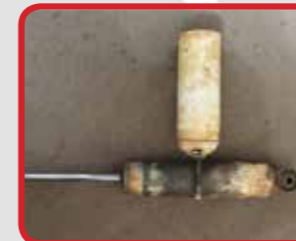
Broken Dust Cover
